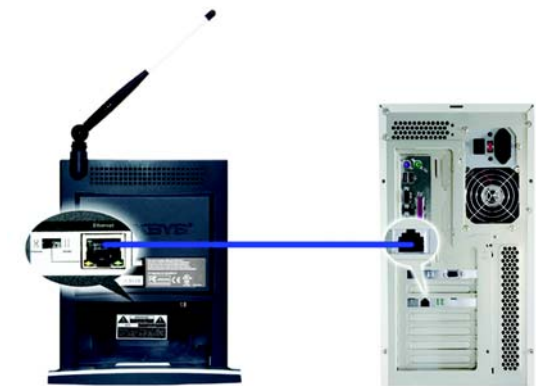
Figure 3-1: Connect the Ethernet Network Cable
